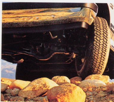
Bronco's rugged Twin-Traction Beam independent front suspension lets each front wheel step over bumps individually for a smoother ride.
