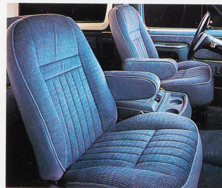
Bronco XLT Crystal Blue interior with optional Captain's Chairs featuring tip/slide mechanism for easy rear-seat entry and exit.
