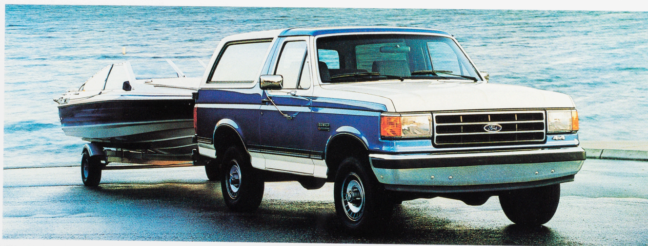
Bronco XLT with optional Trailer Towing Package, 5.0L engine and 4.10 rear axle ratio (automatic overdrive transmission) has a towing capacity of 7,800 pounds.
