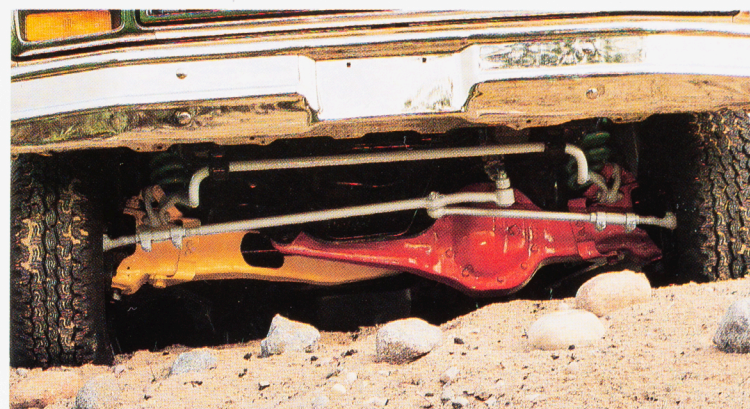
Twin-Traction Beam independent front suspension.
