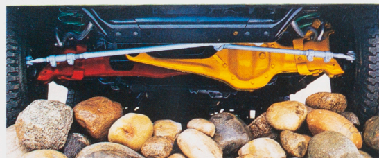
Twin-Traction Beam independent front suspension smooths out the bumps.
