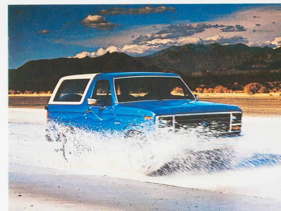
At Ford's Arizona Proving Grounds, extensive corrosion testing includes a salt bath, which exposes all areas of Bronco's underbody and engine compartment to a corrosive spray.
