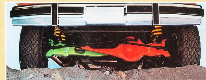
**Tough new Twin-Traction Beam independent front suspension** eases wheels over bumps separately to cushion the vehicle, smooth the going, and improve off-road control. It's smooth on the road—tough off the road.
