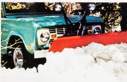
Snowplow Blade may be adjusted to various heights and angles (with kit) from inside the cab.
