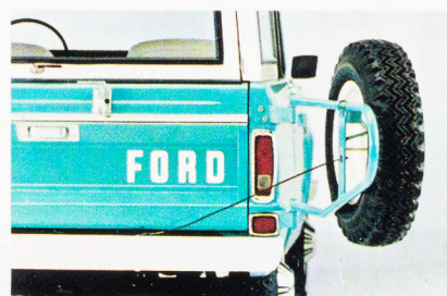
Swing-Away Spare Tire Carrier gets the tire out of the way for more cargo area, easier access.
