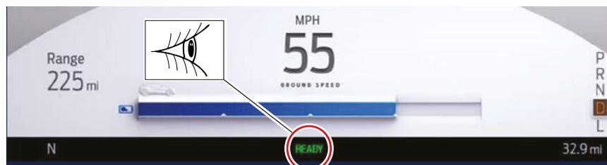
2. If the vehicle READY light is on, press the engine start/stop button to turn off the ignition.
